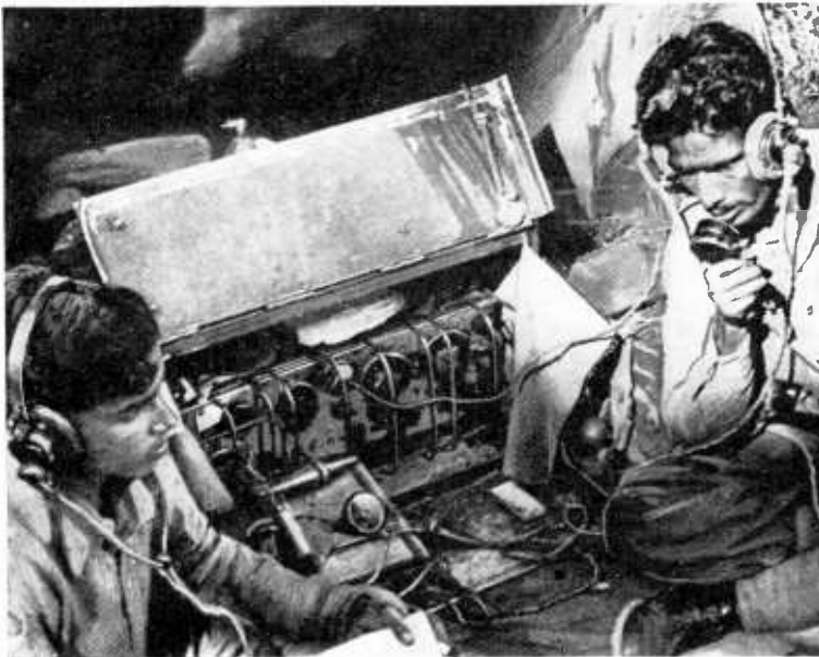
INDIAN SIGNALS. The general-purpose low-power No. 22 transceiver, which has facilities for both 'phone (5W) and CW (15W), in use in the Burma campaign. Men of the Fifth Indian Division are operating the set which has a frequency coverage of from 2-8 Mc/s.
